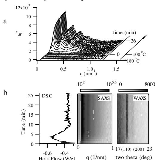
**Figure 1.** Time-resolved simultaneous WAXS/SAXS/DSC measurements during the crystallization at 100°C. Intensity graduations of SAXS and WAXS are in logarithmic and in linear scales, respectively.
