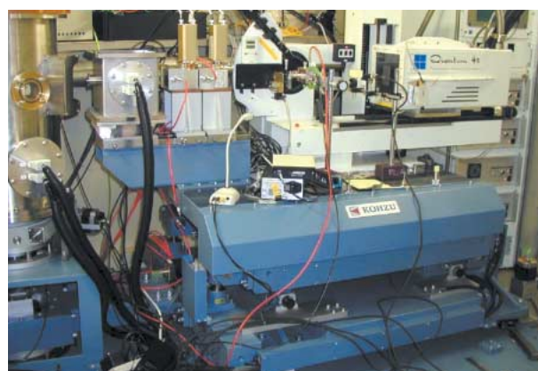
Figure 3 A new optical bench of BL-6A specifically designed for MAD experiments using a CCD detector (ADSC Quantum 4R).
