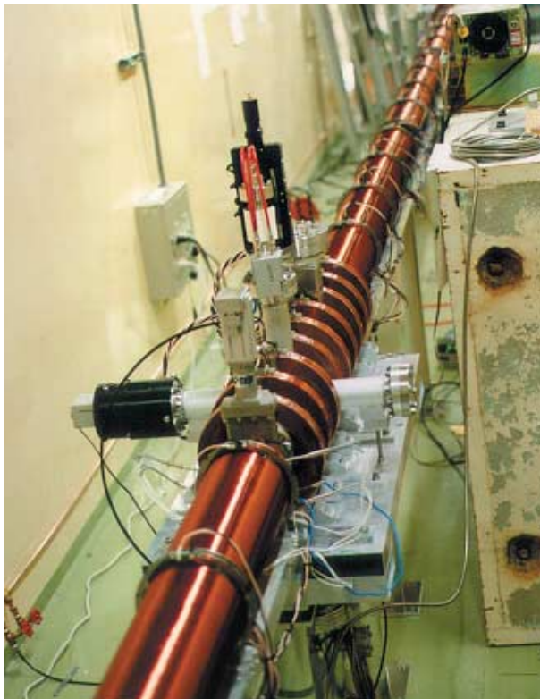
Figure 4 The Helmholtz section of the slow positron beamline. From the upstream to downstream, a gate valve, a screen monitor with MCP for the slow positron beam, a CCD camera, an ion pump (60 l/s), an electrode for Penning trap were installed.
