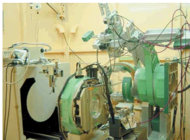
Figure 2 Seven circles diffractometer (7C-XRD, Huber, backward) and imaging plate diffractometer (Rigaku, front) equipped in BL-1A.
