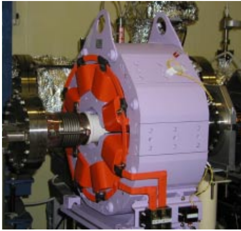
Figure 20 Photograph of the pulsed octupole magnet installed in the PF ring.
