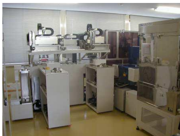
Figure 10 The protein crystallization robot as installed in the extended Structural Biology Building.
