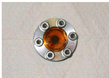
Fig.1: Np sample disc sealed in a container, where the sample was triple sealed by two resin and Capton foil.
