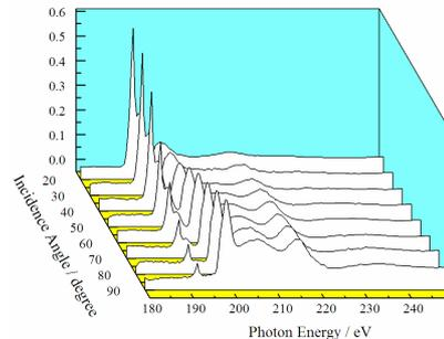
Figure 1. Polarization dependence of B K-edge NEXAFS spectra of *h*-BN/Ni(111). Incidence angle of x-ray is defined as the angle between surface normal and electric vector  $E$  of linear polarized x-ray.
