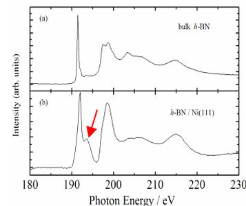
Figure 2. B K-edge NEXAFS spectra of bulk *h*-BN (curve a) and *h*-BN/Ni(111) at 55° incidence (curve b).
