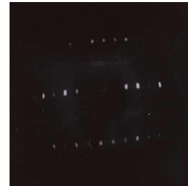
Fig.1 LEED pattern of Si(111)5x2-Gd surface. The pattern indicates clearly that the obtained surface consists of single domain. The faint streaks suggest that the surface has actually x2 periodicity.
