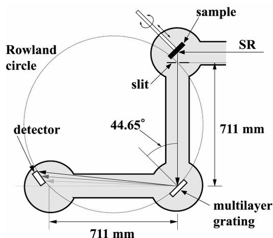
Fig. 1 Schematic layout of the spectrometer.
