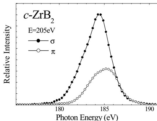
Fig. 3 B 1s emission spectra from ZrB<sub>2</sub>.
