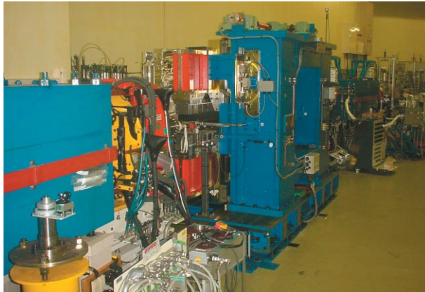
Figure 16 A photograph of MPW#05 as installed in the 2.5 GeV PF storage ring.
