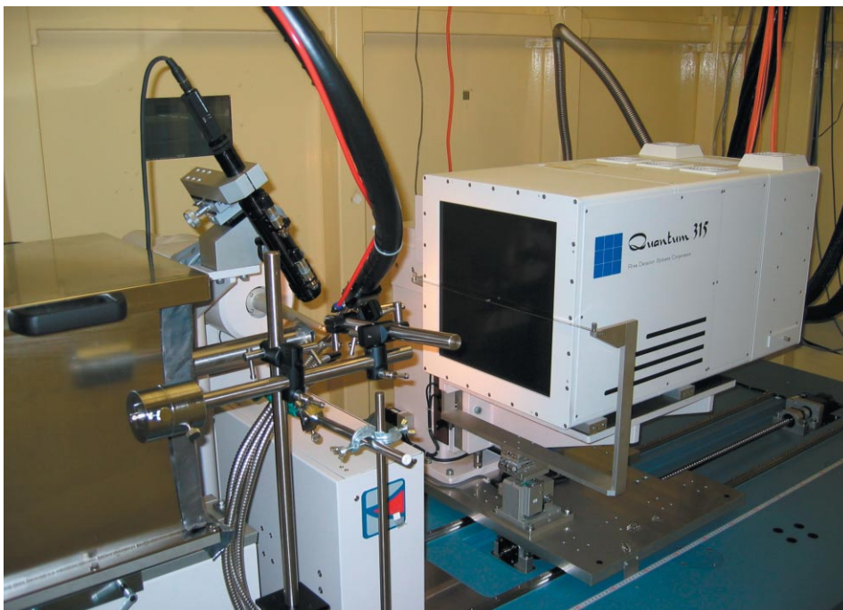
Figure 3 CCD detector (Quantum 315) on the experimental base.
