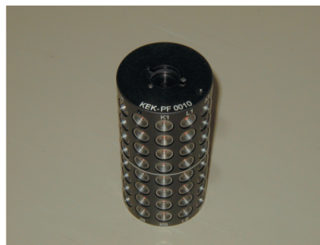
Figure 11 A crystal cassette developed by Stanford Synchrotron Radiation Laboratory.
