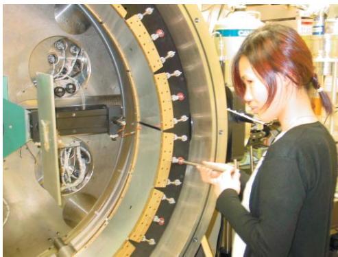
Figure 1 Metta Setyabudi, a Ph.D student at Monash University, sets up a polymer sample for a small and wide-angle X-ray scattering experiment in the ANBF diffractometer.
