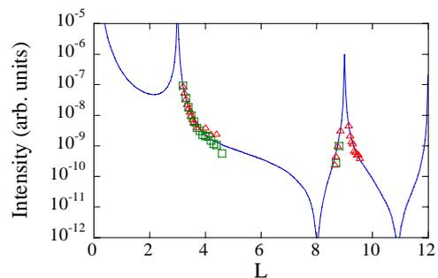
Fig.1 Intensity along 00 rod from Si(111)-6x1-Ag surface. Open triangles and open squares indicate the intensities with the wavelength of 0.86Å and 1.2Å, respectively. Solid line is the calculated intensity on assumption of Collazo-Davila model.
