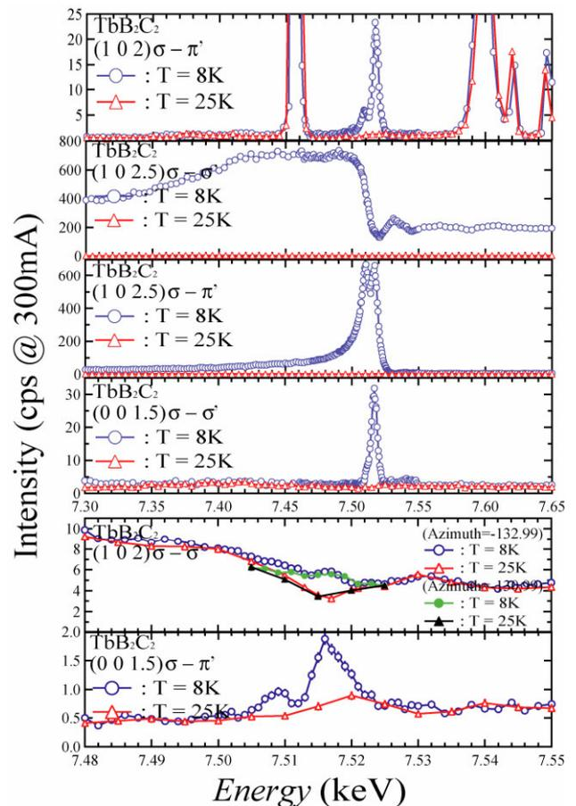
Fig. 1 Energy dependences of all the observed reflections at  $H=12000$  Oe.
