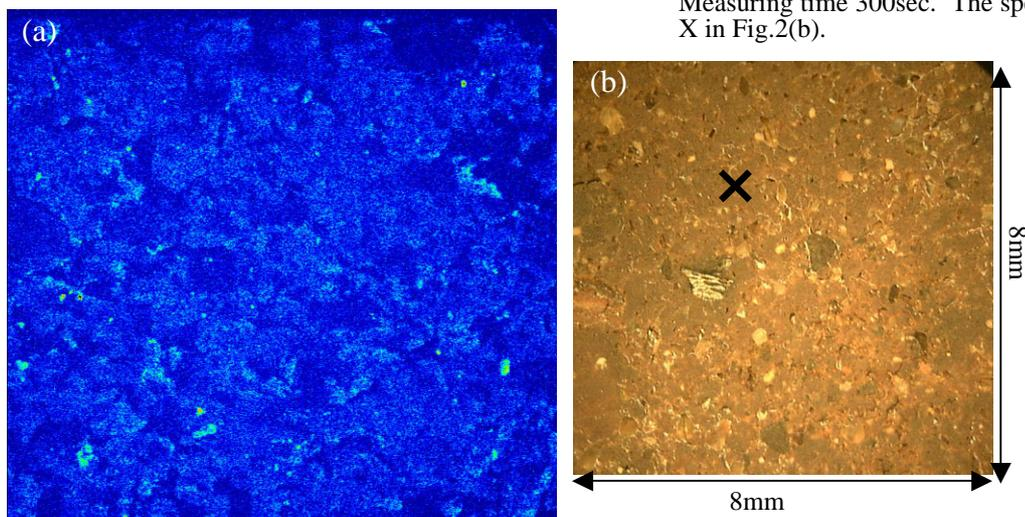
Figure 2 (a) X-ray image of earthenware obtained with white X-rays. Beam size 8mm (H) × 0.2mm (V). Exposure time 70 msec. The image mainly represents a map for iron. (b) Optical microscope photo of the viewing area.
