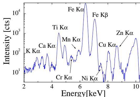
Figure 1 XRF spectra of earthenware, measured with monochromatic X-rays prior to the imaging experiments with white X-rays. Incident X-ray energy 10keV. Measuring time 300sec. The spectra were taken at position X in Fig.2(b).
