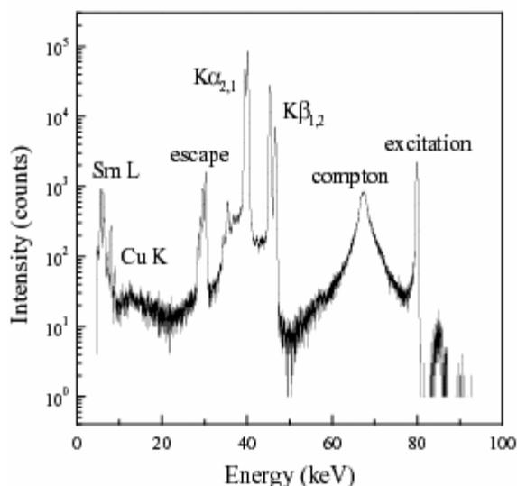
Figure 1 High-energy XRF spectrum of  $\text{SmF}_3$ .
