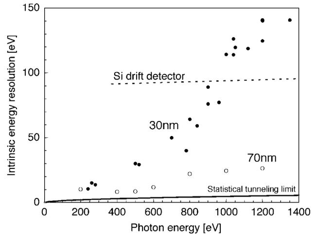
Fig. 1 Energy resolution (fwhm) of an  $100\mu\text{m}$ -square detector as a function of photon energy. The closed and open circles show data for different layer structures of superconducting proximity electrodes.
