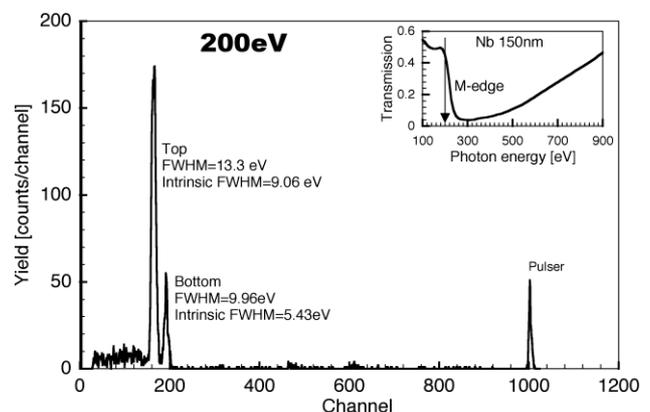
Fig. 2. Pulse height spectrum for X-rays of 200 eV. The best energy resolution is 10 eV.
