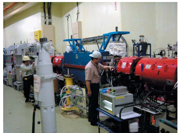
Figure 9 Coordinate survey using the laser tracker system.
