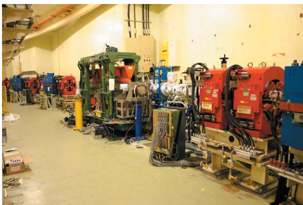
Figure 8 Images before (top) and after (bottom) the rearrangement of the quadrupoles around MPW#16. Free spaces of 2 m long are created at either end of MPW#16.
