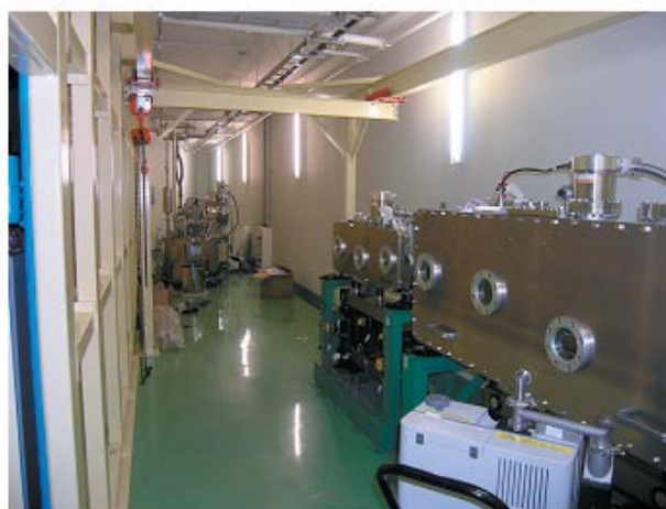
Figure 11 Monochromator and mirror chambers installed in the optics hutch.
