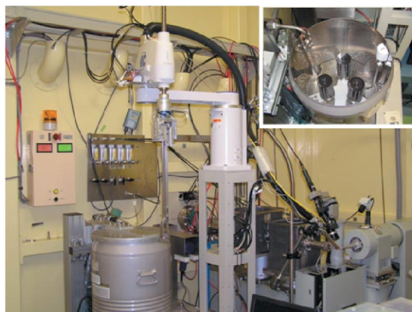
Figure 12 Overview of the sample exchange robot installed at AR-NW12A. The inset shows an inside view of the Dewar in which three SSRL cassettes are held in place.
