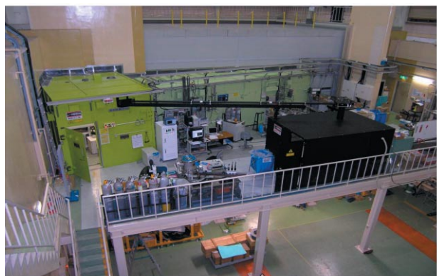
Figure 2 The experimental hutch (green) and laser hutch (black). The hutches are connected by a black pipe for transport of the laser beam.
