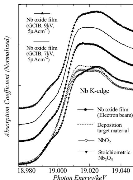
Fig. 1. Nb K-XANES of Nb oxide thin films, which were formed by the GCIB assisted deposition and electron beam deposition together with those of various Nb oxides.
