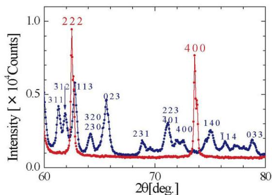
Figure 2 X-ray powder diffraction patterns for monoclinic and cubic zirconia.
