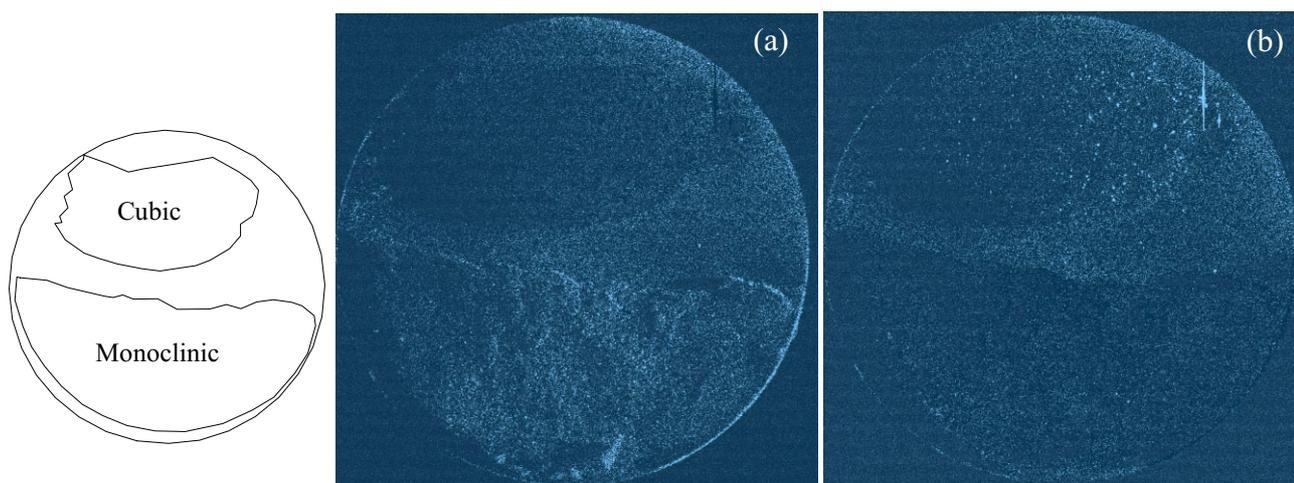
Figure 1 (left) A schematic drawing of the sample. The sample consists of monoclinic and cubic zirconia. Figure 3 (right) (a) monoclinic zirconia image, (b) cubic zirconia image. The images were obtained from XRD images collected at two different energies of 6787eV and 6889eV, which correspond to Bragg reflections of cubic (400) and monoclinic (140), respectively.
