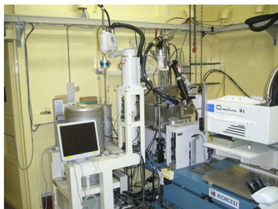
Figure 6 Inside view of the experimental hutch of BL-17A. The sample exchange robot (SAM system) is located beside the diffractometer.
