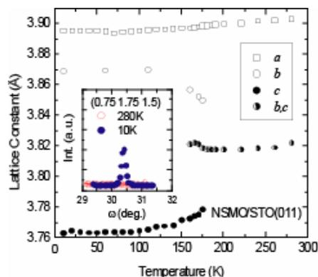
Fig.1 Temperature dependence of the lattice parameters. (inset) Intensity distribution around  $(3/4\ 7/4\ 3/2)$  measured at 10K and 250K.
