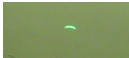
Figure 2 A beam shape at the entrance of the experimental hutch. on the beamline BL18B.
