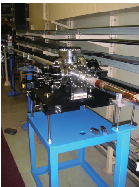
Figure 20 First slit in the large dispersion section to limit energy spread.
