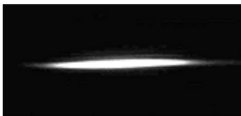
Figure 41 Qualitative image of the electron beam observed using the focusing system.
