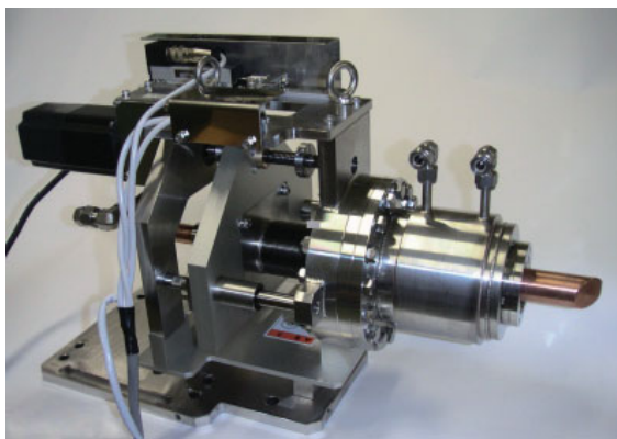
Figure 3 Photograph of the movable SR mask.
