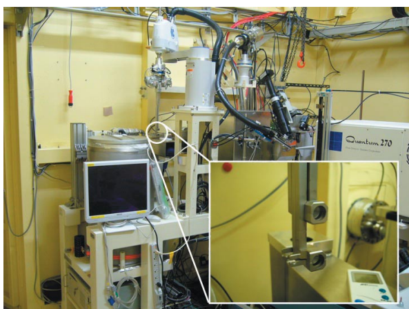
Figure 7 Sample exchange robot installed at BL-17A. The inset shows a magnified image of the double tong system developed at KEK-PF, which improves sample exchange throughput compared to using a single tong.
