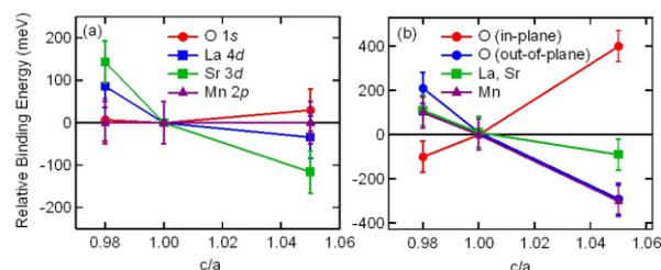
Fig. 1: Binding-energy shifts of each core level in LSMO thin films. (a) Experimental values determined by photoemission spectroscopy. (b) Calculated values determined from the effect of  $\Delta V_M$ .
