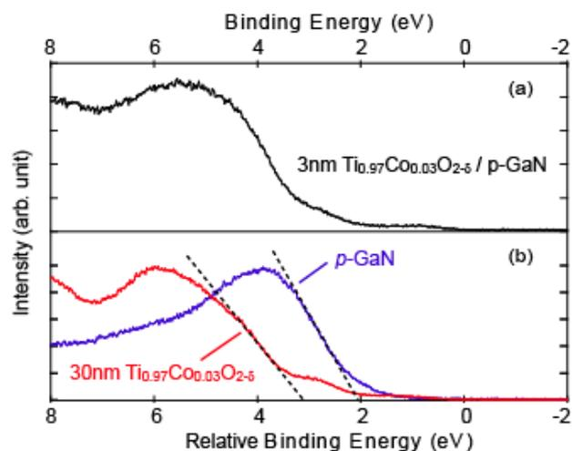
Figure 1 Valence band spectra of  $\text{Ti}_{1-x}\text{Co}_x\text{O}_{2.8}/p\text{-GaN}$
