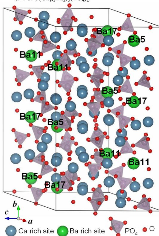
Fig.2. Refined crystal structure of Ba-substituted  $\alpha$ -TCP,  $(\text{Ca}_{1-x}\text{Ba}_x)_3(\text{PO}_4)_2$  ( $x=0.15$ )
