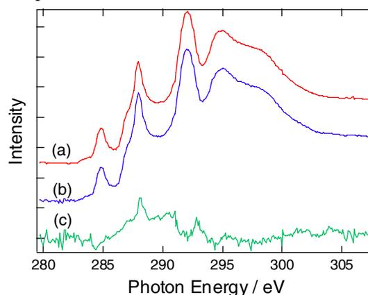
Fig. 1 C 1s XAS spectra of (a) initial MEA, (b) 10,000 cycle-tested MEA and (c) difference between (a) and (b), whose magnitude is enhanced 5 times.
