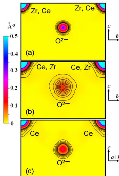
**Fig. 2.** Parts of electron density distributions on the (100) planes of (a)  $\text{Ce}_{0.12}\text{Zr}_{0.88}\text{O}_2$  and (b)  $\text{Ce}_{0.5}\text{Zr}_{0.5}\text{O}_2$ . (c) A part of electron density distribution on the (110) plane of  $\text{CeO}_2$  with black contours in the range from  $4.0$  to  $20.0 \text{ \AA}^{-3}$  ( $2.0 \text{ \AA}^{-3}$  step) at  $299 \text{ K}$  ( $1/2 \leq z \leq 1$ ).
