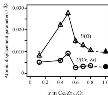
**Fig. 1.** Composition dependence of isotropic atomic displacement parameters of Ce and Zr atoms  $U(\text{Ce, Zr})$  and O atoms  $U(\text{O})$  in tetragonal  $\text{Ce}_x\text{Zr}_{1-x}\text{O}_2$  solid solutions and cubic  $\text{CeO}_2$  ( $x=0.12-1$ ).
