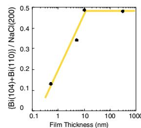
Fig. 3 The film thickness dependence of the peak intensities of the Bi (104) and (111) peaks
