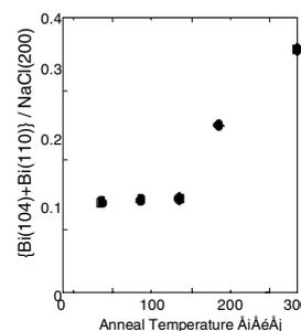
Fig. 2 The peak intensities of the Bi (104) and (111) peaks of the annealed 0.5 nm-thick-films.
