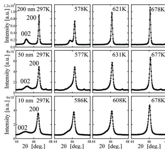
FIG. 1 Peak profiles of 200 and 002 reflections in PST7/3 nanoparticles at various temperatures and particle sizes.
