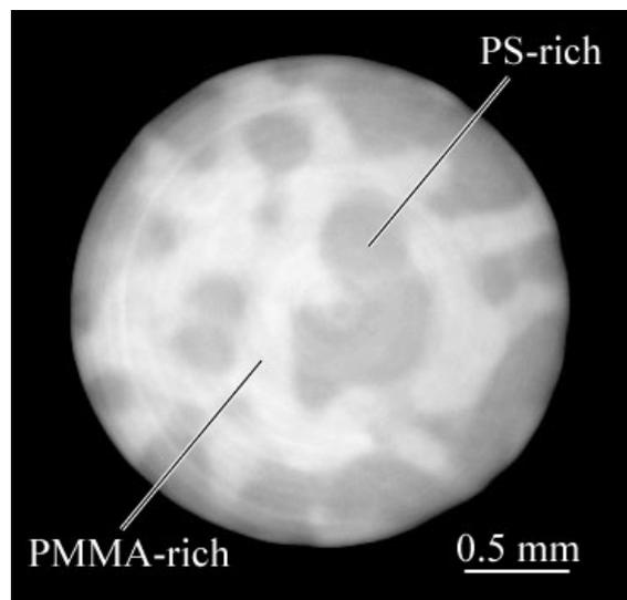
Fig. 1 X-ray phase tomogram of a PS/PMMA blend with a phase-separation structure. The total scan time was only  $0.5 \text{ s}$ .
