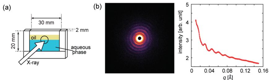
Figure 1 Inspection of aggregate generation: (a) Experimental setup. (b) SAXS image and its azimuthal average.
