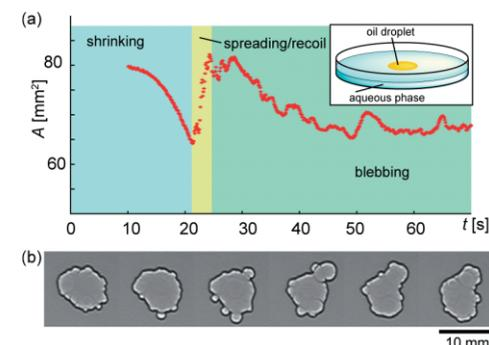
Figure 2 Manner of droplet deformation: (a) Change in apparent area,  $A$ , of an oil droplet. Inset: Schematic representation of experimental setup. (b) Blebbing motion observed in late stage of droplet deformation. Snapshots start from 48 s and were taken every 2 s.
