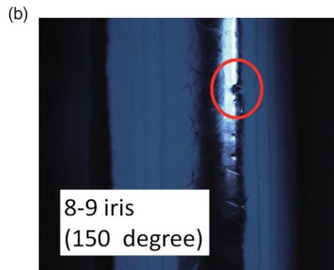
Figure 16 (a) X-ray mapping data at  $E_{acc} = 13.9$  MV/m. (b) Picture of inner surface of cavity. A tip was found at the iris between 8-cell and 9-cell.
