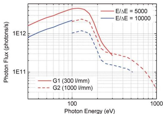
Figure 6 Photon flux estimated with analytical calculations when the exit slit is adjusted to achieve the energy resolution ( $E/\Delta E$ ) of 5,000 and 10,000 [1].
