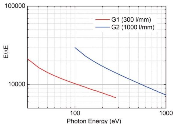
Figure 5 Energy resolution ( $E/\Delta E$ ) in the simultaneous scan of M2 and VLSG, estimated with analytical calculations [1].
