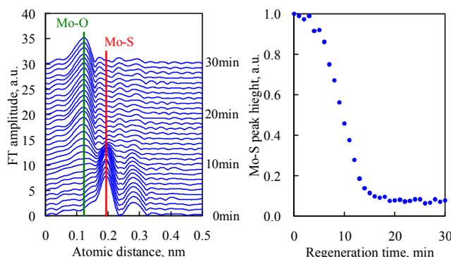
Fig. 1: FT of Mo K-edge EXAFS and regeneration time dependence of Mo-S-peak-height.
