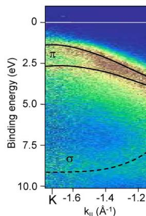
Fig. 2: Angle-resolved photoelectron intensity distribution ( $h\nu=50 \text{ eV}$ ) of sample B, after an annealing at 650 °C for about 120 min in total.
