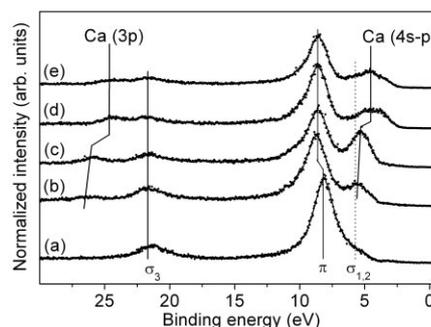
Fig. 1: Spectra ( $h\nu=70 \text{ eV}$ ) of sample A at the  $\Gamma$  point obtained *prior* (a) and after (b) Ca deposition, as well as after a short (5 min, (c)), extended (30 min, (d)) and long (90 min, (e)) annealing at 400 °C.
