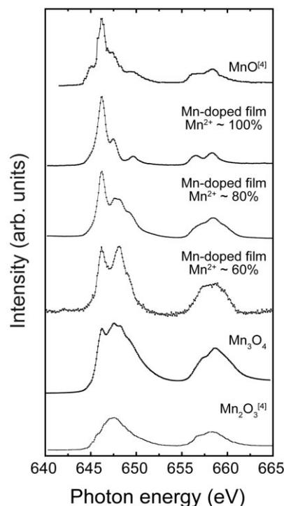
Fig. 1 Mn- $L_{2,3}$  XANES spectra of Mn-doped  $\text{Ga}_2\text{O}_3$  films with various-mixed valence states, compared with those of MnO [4],  $\text{Mn}_3\text{O}_4$ , and  $\text{Mn}_2\text{O}_3$  [4].
