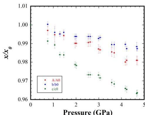
Fig.1 Normalized lattice parameters at T=300 °C.
