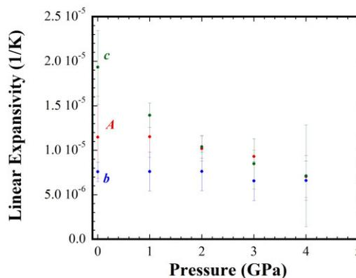
Fig.2 Linear expansivities as a function of pressure.
