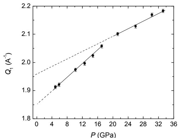
Fig. 2. Scattering vector corresponding to first ADP as a function of pressure.
