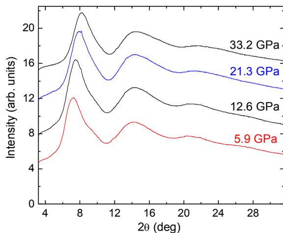
Fig. 1. Diffraction patterns of amorphous  $Zr(WO_4)_2$  at different pressures.
