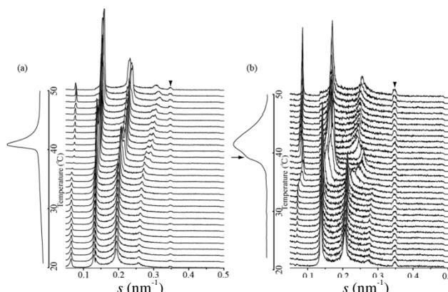
Figure 1. DSC heating thermograms and corresponding temperature-resolved SAXD patterns of the DPPG/chol liposome (a) in the absence and (b) in the presence of cyd. The arrow in (b) indicates the newly appeared transition (see Text). The scattering vector is defined as  $s=2\sin\theta/\lambda$ , where  $2\theta$  is the scattering angle. Arrowheads indicate the reflection from the kapton film.
