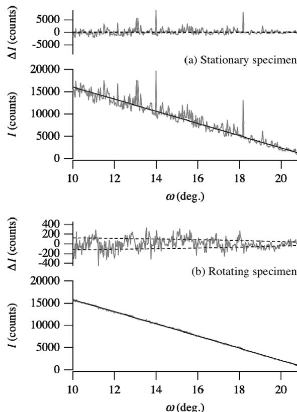
**Fig. 1**  $\omega$ -scan intensity profile of Si 111-reflection measured for (a) stationary and (b) rotating specimens. Observed and fitted profiles are shown as gray and black lines in the lower panels. The broken lines in the upper panels show the standard deviation predicted from counting statistics.
