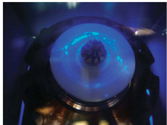
Figure 31 Oil (fluorescent parts with black light) from a helium compressor on a Teflon disk of the first-stage turbo-expander.
