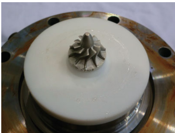
Figure 30 Oil from a helium compressor on a Teflon disk of the first-stage turbo-expander.
