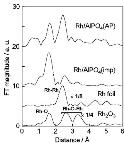
Figure 1 Fourier transformed Rh K-edge EXAFS for 0.4 wt%  $\text{Rh}/\text{AlPO}_4$  as prepared by wet impregnation and arc-plasma process.
