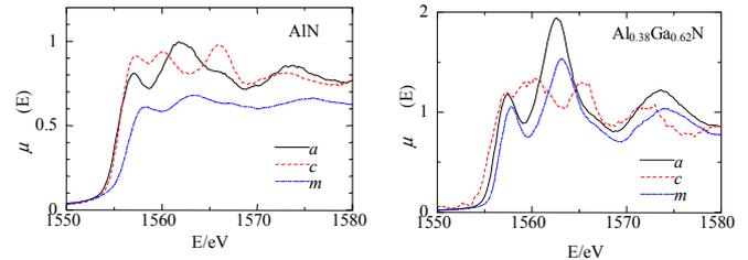
Fig. 1 Al *K*-edge XANES of *a*-, *c*-, *m*-directions of *m*-plane AlN (2.1 $\mu$ m thick) and Al<sub>x</sub>Ga<sub>1-x</sub>N (140 nm thick,  $x = 0.38, 0.58$ ).
