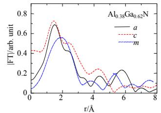
Fig. 2 Fourier transforms of *a*-, *c*-, *m*-directions of *m*-plane AlN (2.1 $\mu$ m thick) and Al<sub>x</sub>Ga<sub>1-x</sub>N (140 nm thick,  $x = 0.38, 0.58$ ).
